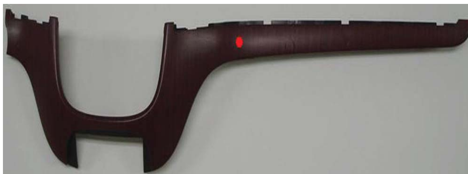
Figure 3 Complex automotive interior part showing the location where the residual stress distribution was measured. [Color figure can be viewed in the online issue, which is available at www.interscience.wiley.com .]
